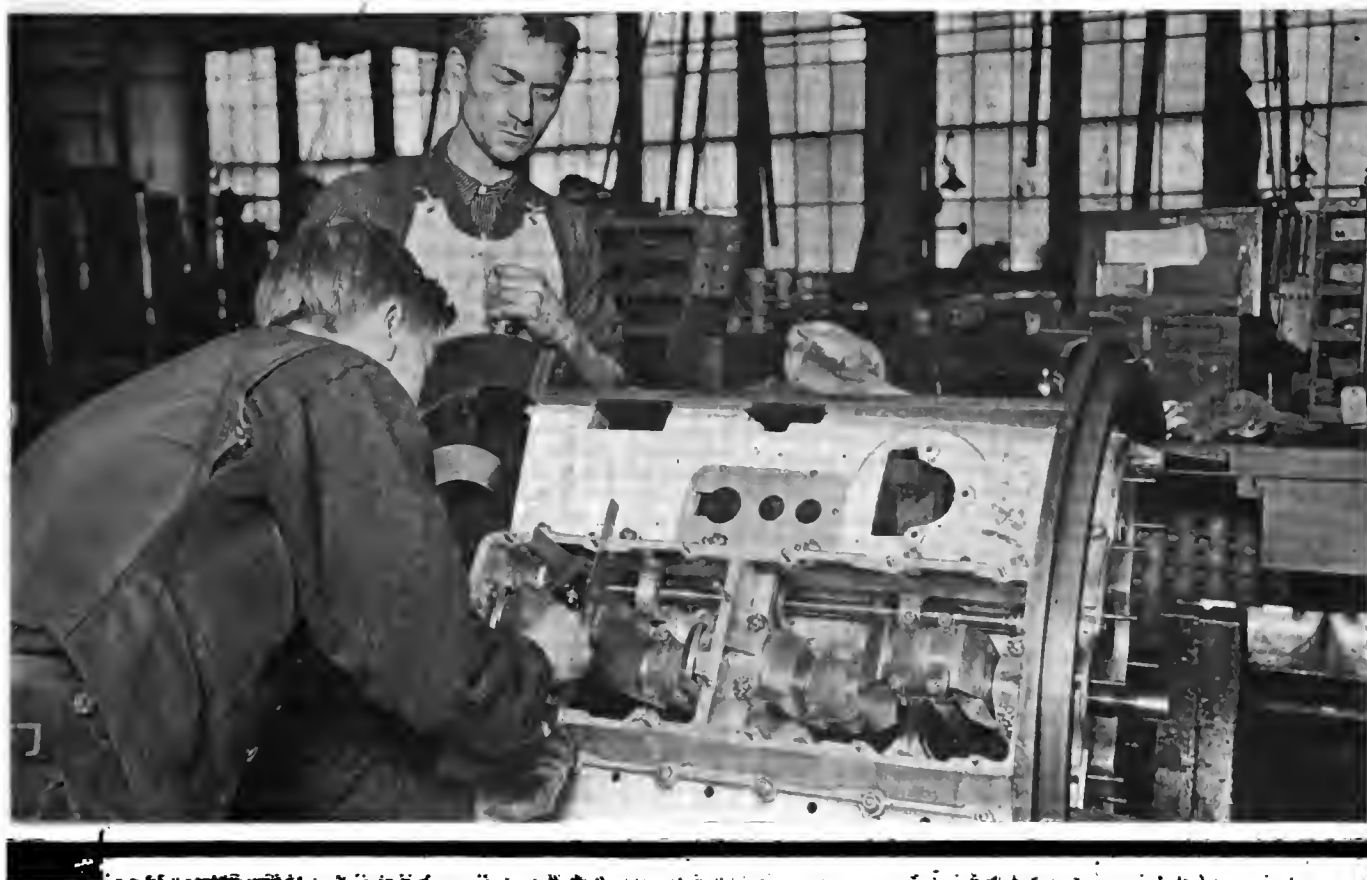
ERECTING MOTORS AT THE PACKARD PLANT, ILLUSTRATING THE USE OF SPECIALLY CONTRIVED STANDS
